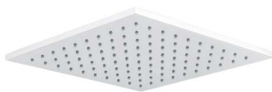
Square Shower Head with 1/2" Connection 250 x 250 x 8 mm Min. Operating Pressure 0.5 bar LP
